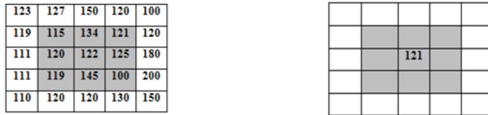
Figure 3.3 Illustration of median filter (a) Input image (b) Filtered image using median filter showing only the center pixel
