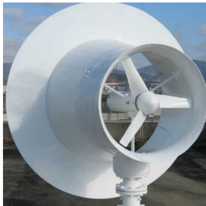
Figure 2-4: A Shrouded wind turbine (Yuji Ohya et al. 2008)
