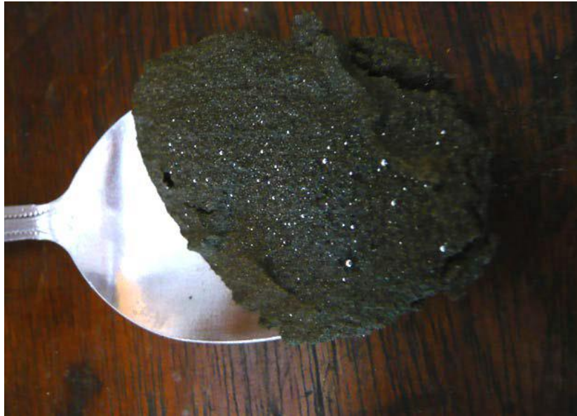
Fig 2.3: Milled gold ore with mercury flour (Source: Appel & Na-Oy, 2014).
