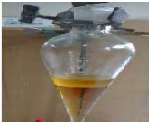
Appendix 13: Methyl esters with upper biodiesel layer and lower glycerol layer.
