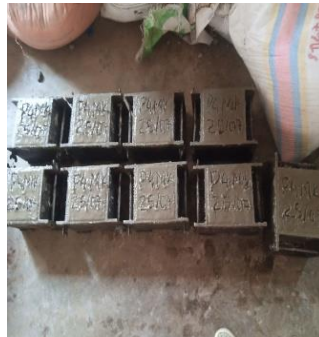
B) Concrete cubes for compressive strength test
