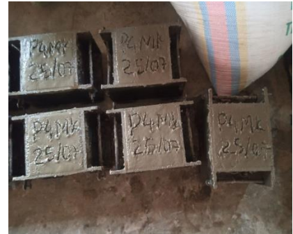
B) Concrete cubes for compressive strength test
