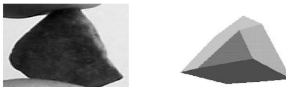
Figure 2.7: Comparisons of an actual aggregate particle with the discrete element representation generated [33]
