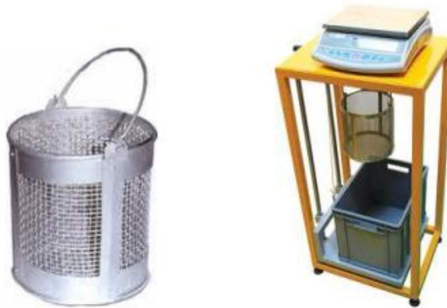
Fig. A.D.4 Wire basket and weight balance
