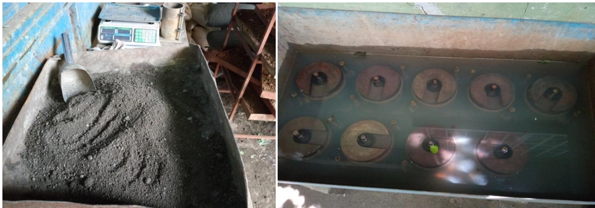
Figure 3:9: Sample preparation for CBR & CBR soaking
