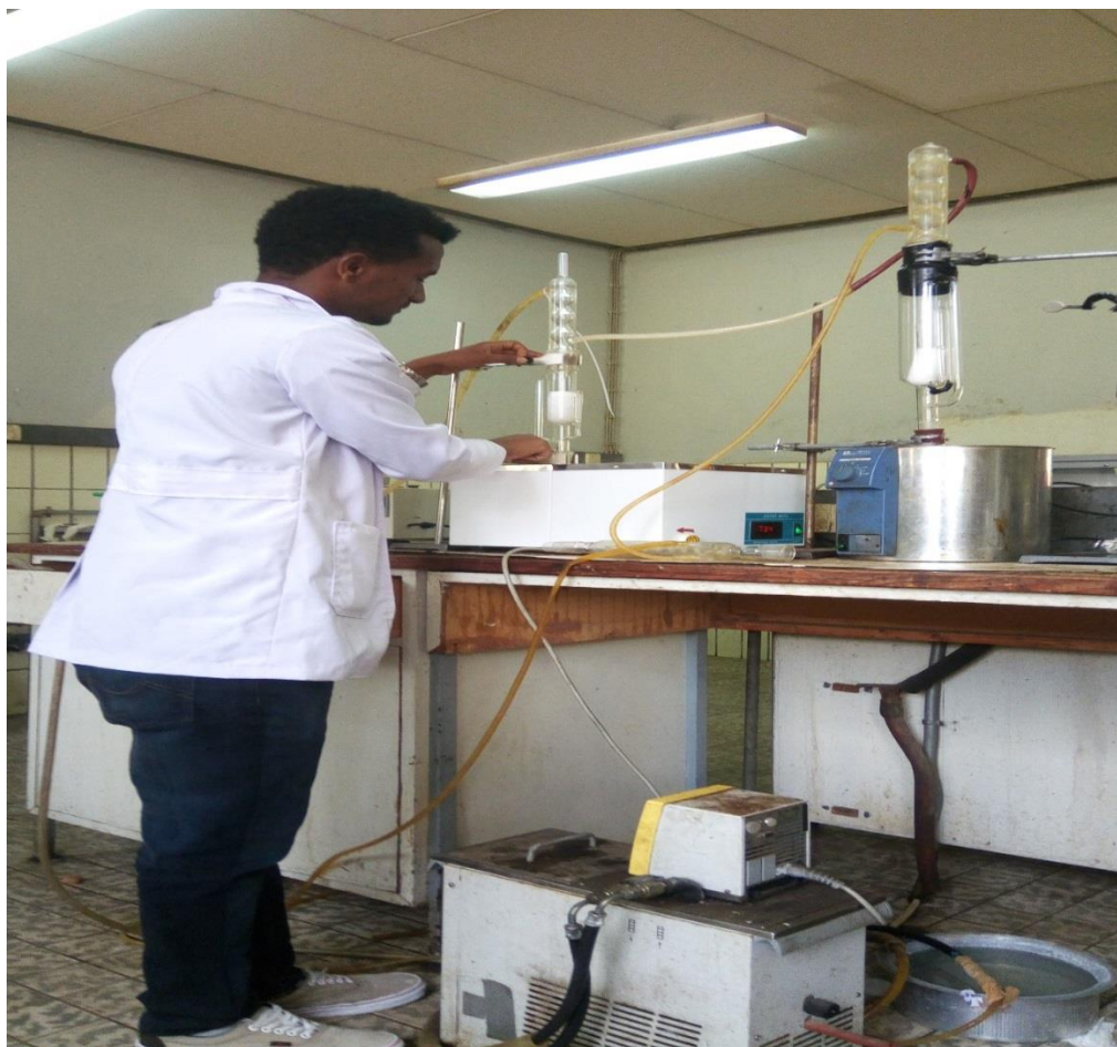
Figure 3.5 laboratory setup of Soxhlet extraction
