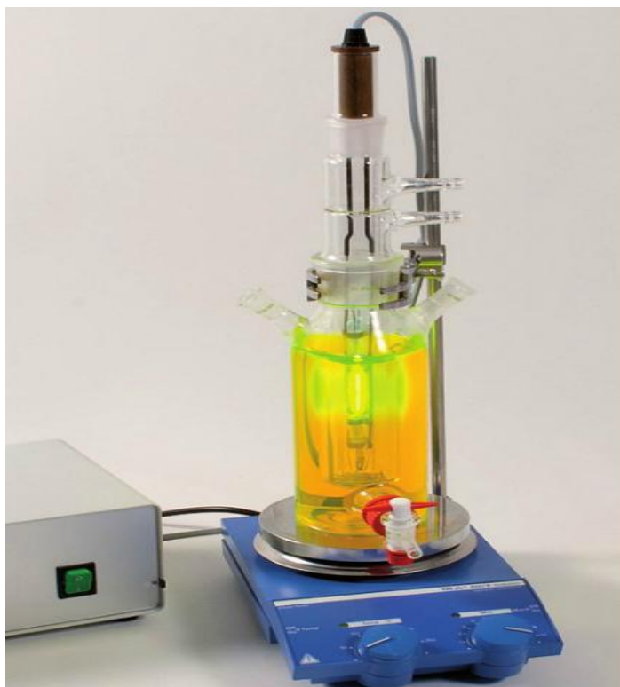
Figure 11: Heraeus medium pressure mercury lamp, photocatalytic reactor
