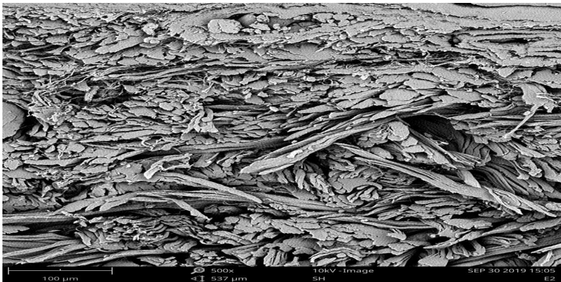
Figure 4.1.d Scanning electron micrographs of the cross-section (x500) of upper crust leather for experimental
