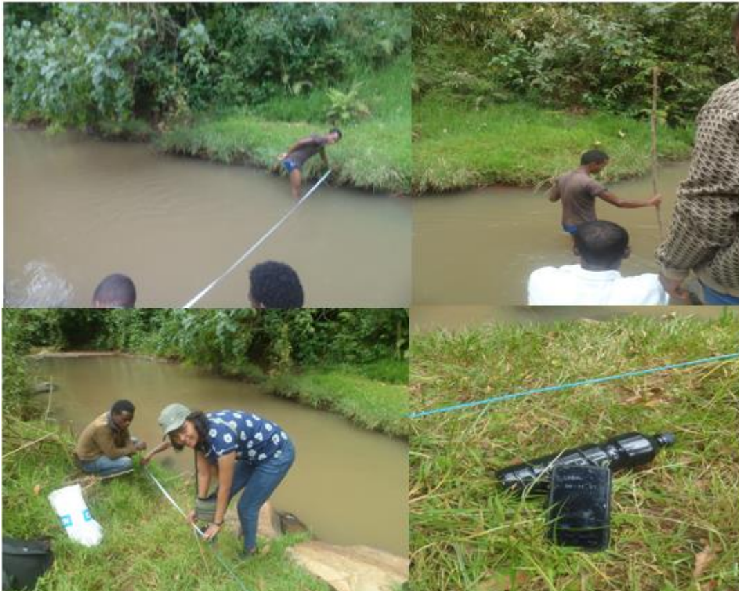
Figure 2: Floating method flow
