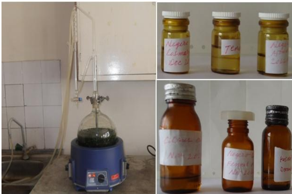
Figure 2.1: Essential oil extracts of plant material using Clevenger-type apparatus
