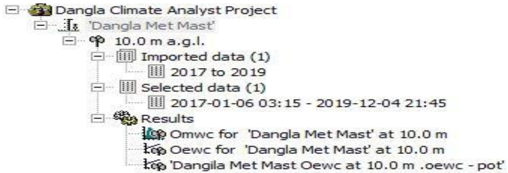
Figure 3.8 WAsP Climate Analyst Setup for wind data analysis and calculating Observed Wind Climate
