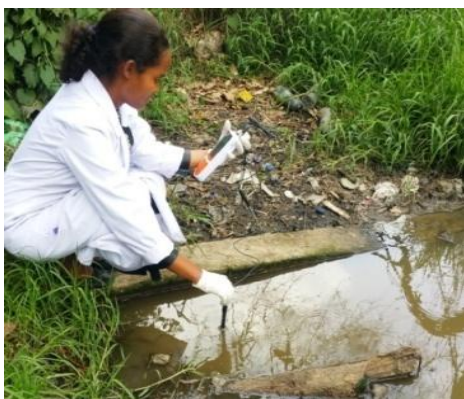
Figure 4. Onsite pH, temperature and conductivity analysis of the raw wastewater at Tikur Anbessa Specialized Referral Hospital at the time of sample collection (Feb-June 2018)
