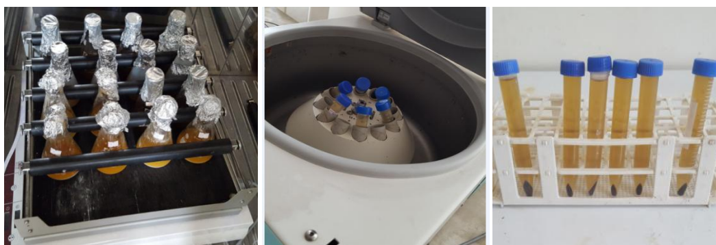
Figure 3-12: Fermentation and centrifugation process
