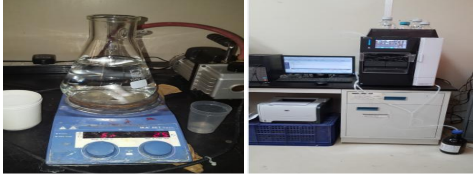
Figure 3-15: HPLC lactic acid determination process
