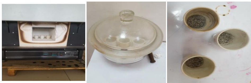
Figure 3-4: Ash content determination process
