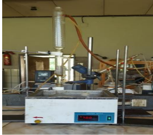
Figure 3-5: Soxlet extraction process
