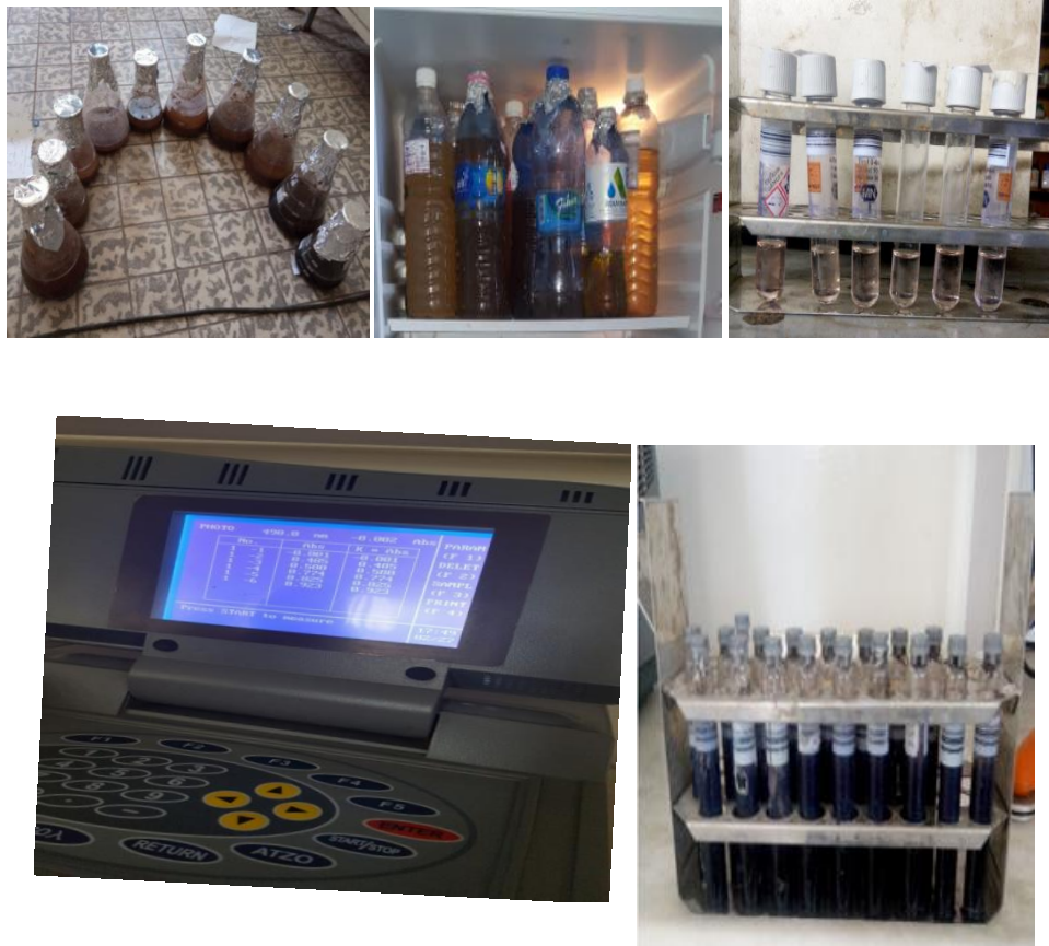
Figure 3-9: Glucose content determination process
