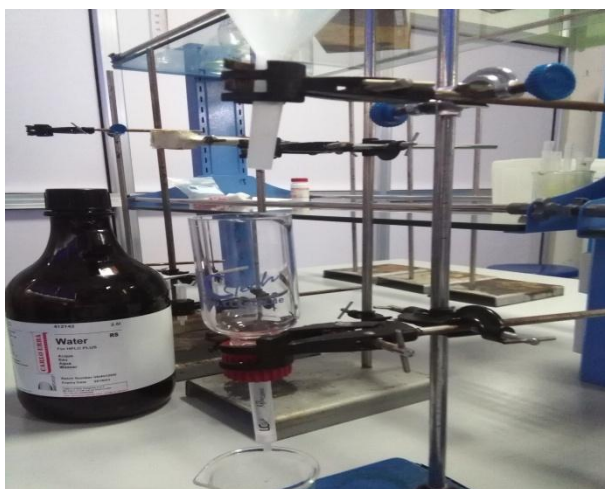
Figure 4.2: Immune affinity column fitted with syringe barrel (Source: Generated during analysis, 2017)
