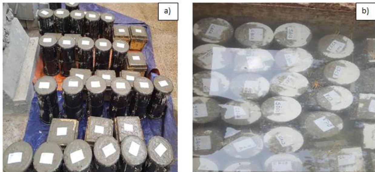
(a) Casting and (b) immersing to tap – water of concrete specimens
