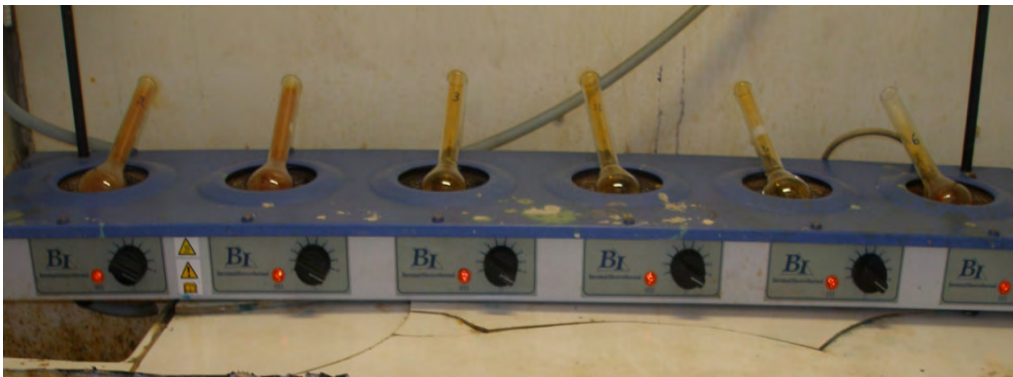
Figure 9: Wet digestion system
