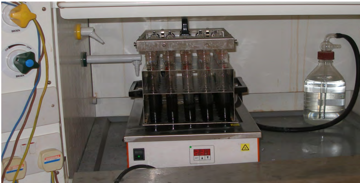
Figure 4: Block digestion system for protein determination
