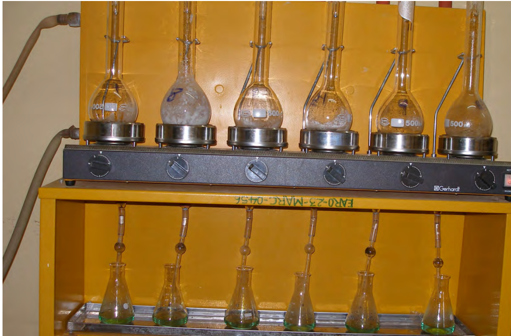
Figure 5: Distillation system for protein determination
