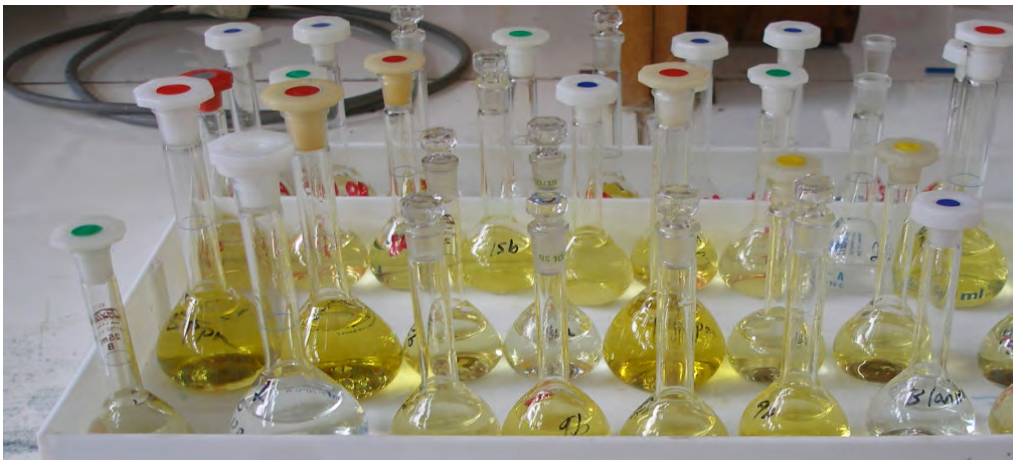
Figure 8: Complex formation for phosphorus determination
