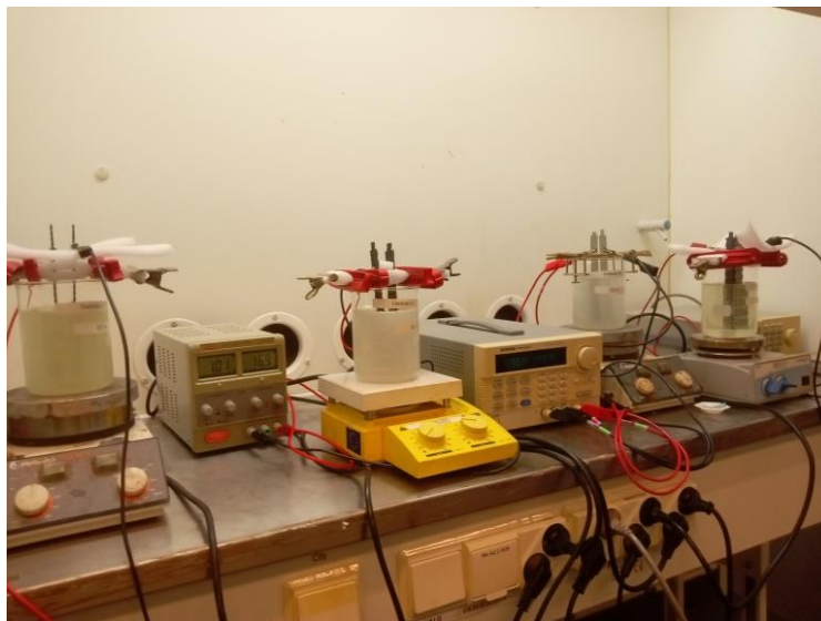
Figure 3.4. The electrochemical oxidation setup used in this study.
