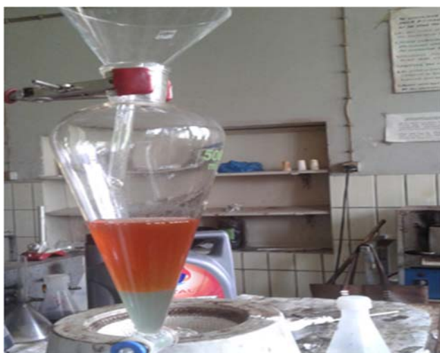
Figure 4.1. Methyl ester sulfonic acid separation in a separating funnel
