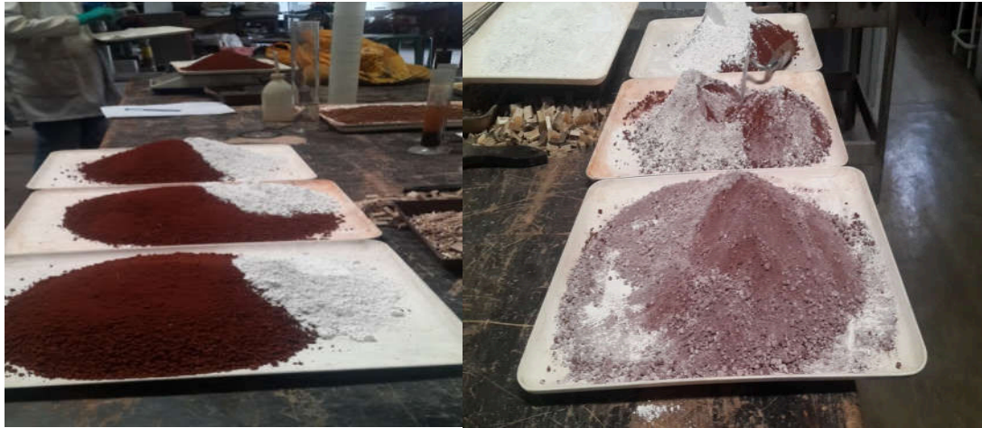
Fig 4.4 Picture of sample blending with lime for compaction in dry state
