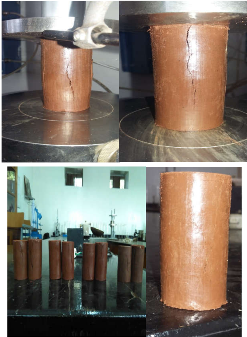
Fig 4.7 Samples in Unconfined Compression test
