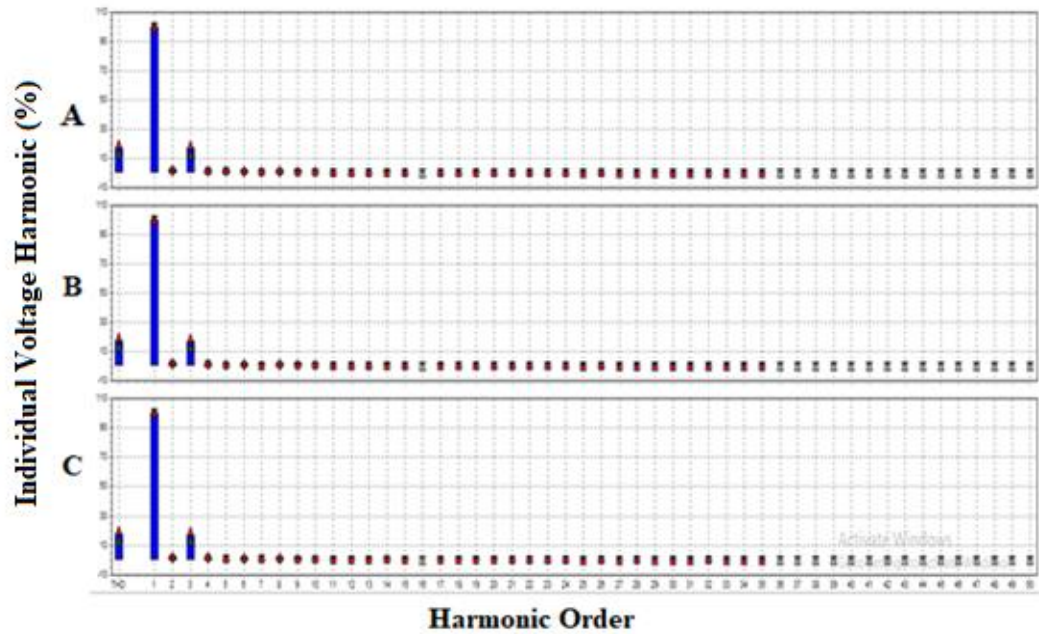
Figure 2.5: Individual voltage harmonic spectrums of wye line
