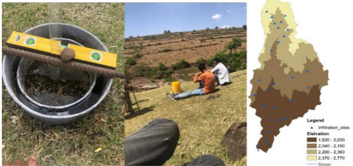
Appendix Figure 7 Infiltration measurements using a double-ring infiltrometer from 36 sampling sites in the Dirima watershed
