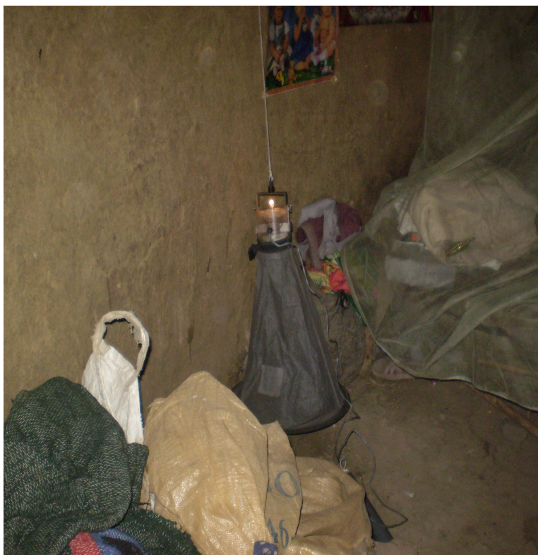
Plate 3. CDC light trap used to collect endophilic and/or endophagic night biting mosquitoes indoors
