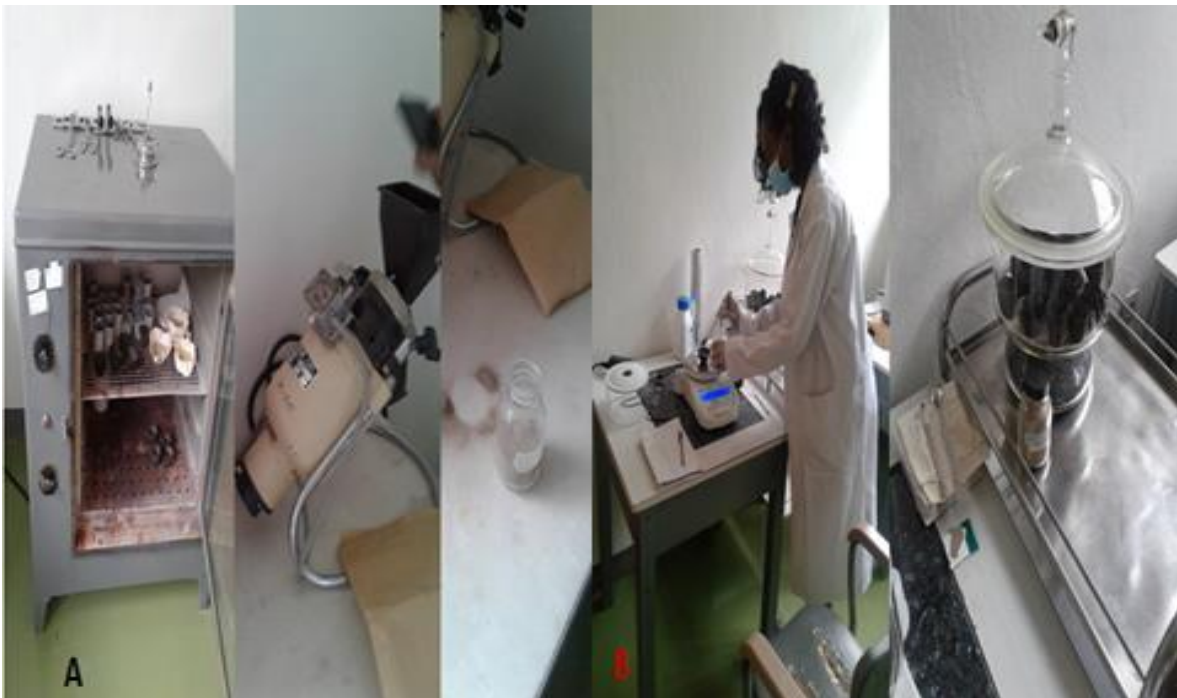
Appendix Figure 4. Some of the materials and steps during chemical analysis at National Veterinary Institute (NVI) Laboratory A) Oven dry machine (Left), Grinder machine(Middle) and grinded sample for analysis(Right) B) Grinded sampling weighing on sensitive balance for further chemical analysis(Left).
