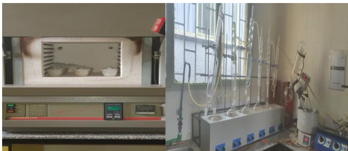
Appendix 5. Picture showing ash determination in the furnace and analysis of crude lipid proximate chemical composition by Soxhlet extractor analysis in the NFALRC laboratory
