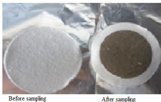
Figure 4. The photo of filter paper before and after sampling at Akaki Kaliti sub-city (Maselitegna sub-site) on October 25, 2017.
