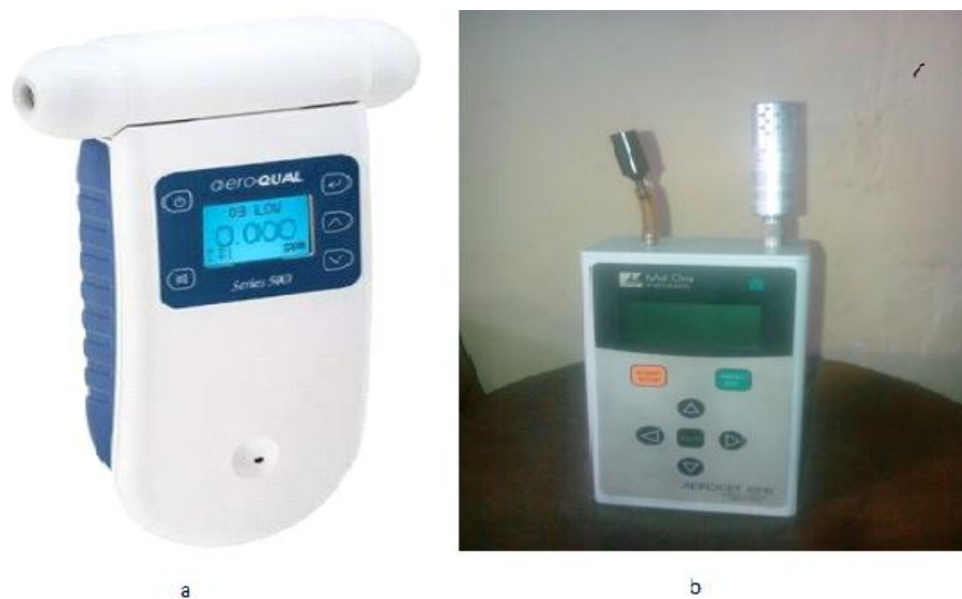
Figure 3. Air sampler device and assembling a) Aeroqual series 500 and b) AROCET531S.
