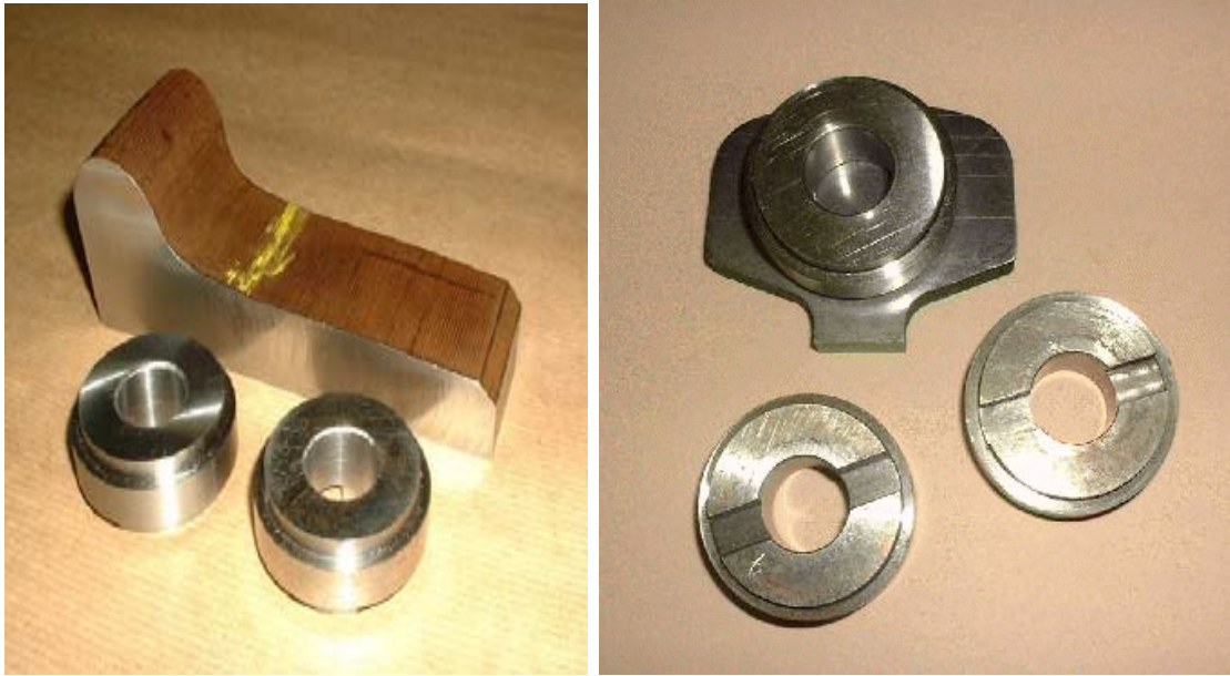
Figure 2.16 Wheel and Rail Disc Specimens taken from wheel and rail [8]
