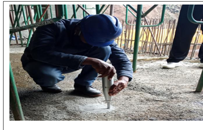
Rebounder hammer reading on floor slab
