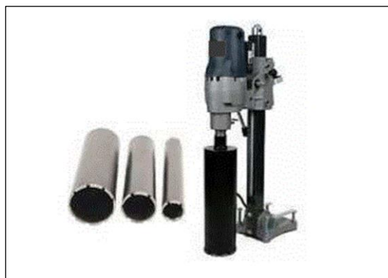
Figure 2.11. Core drilling rig (Maitham Fadhil Abbas Alwash,2017) [26]
