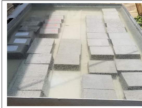
Figure 5.8. Concrete Soaked in water for curing until the age of testing
