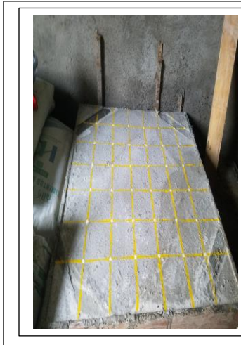
Casted slab and pad prepared for coring
