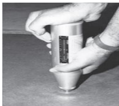
Figure 2.1. Rebound hammer for nondestructive evaluation of hardened concrete
