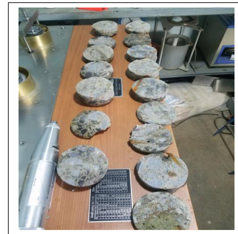
Rebound hammer reading from slab
