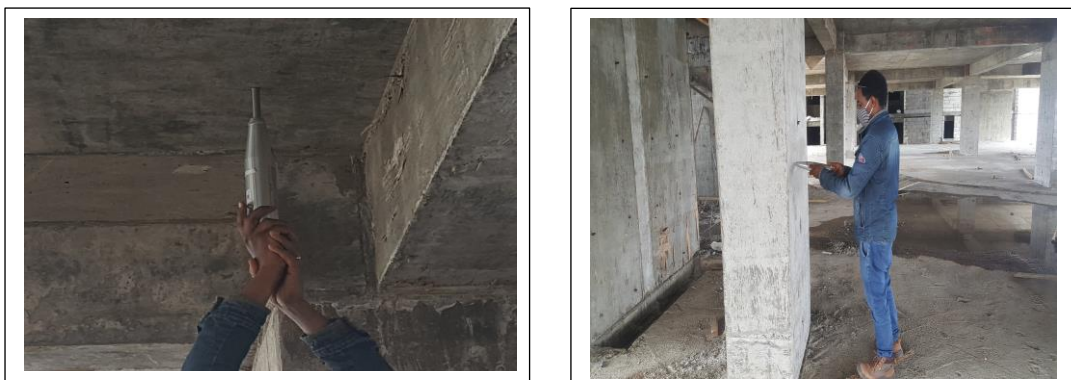
a) Hammer reading from slab
