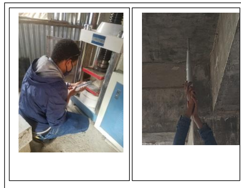
Rebound hammer reading on cube samples
