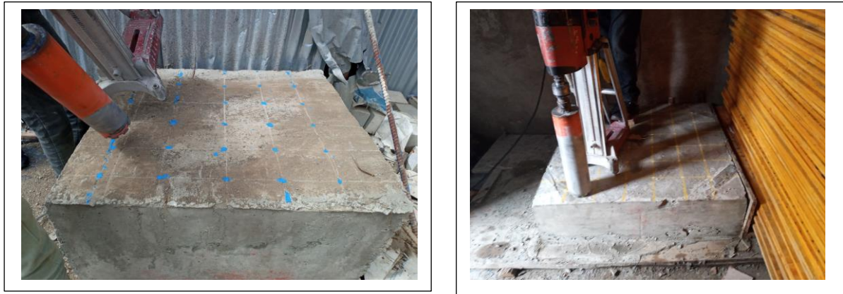
Figure 5.2. Sample preparation for coring (Pictured by researcher)
