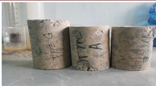
Figure 5.14. Core samples after Testing from Ever grand site
