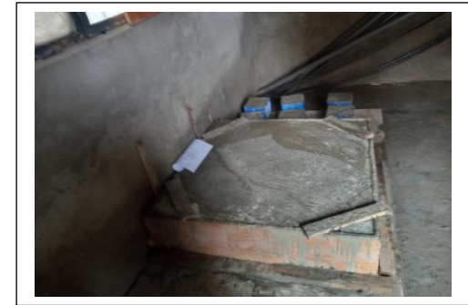
A 1.0m by 1.0m casted slab
