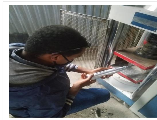
Figure 5.9. Laboratory Schmidt hammer rebound reading
