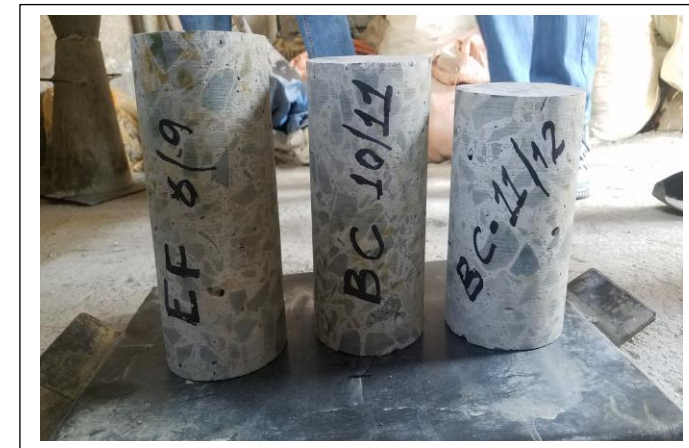
concrete cored trimmed and ready for crushing
