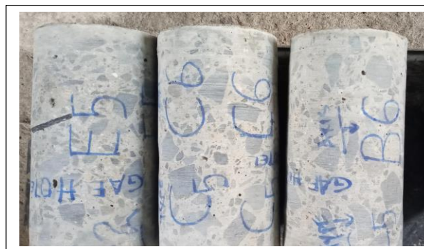
Figure 5.10. Cored sample trimmed and capped and ready for crushing from GAF site
