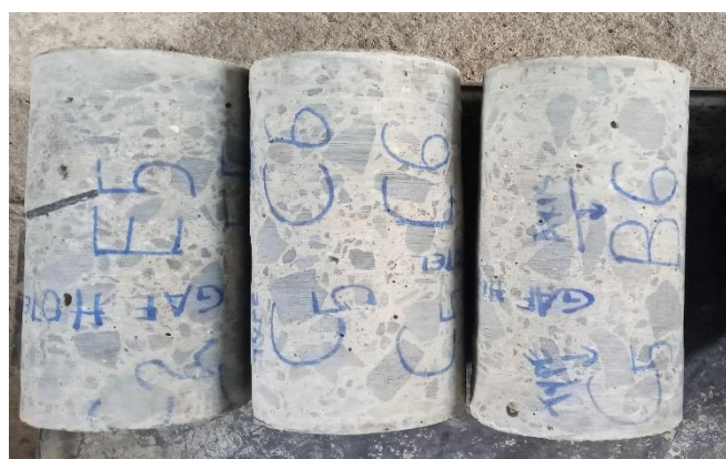
Figure 5.17. Core samples after trimming from GAF site
