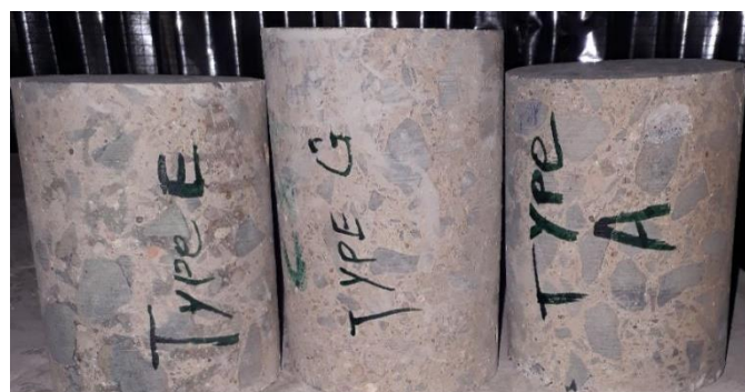
Figure 5.13. Core samples after Trimming from Ever grand site
