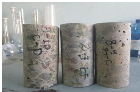
Figure 5.16. Core samples after Trimming from Fedengua site
