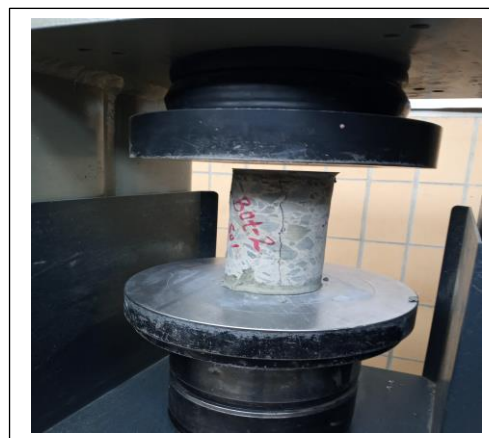
Figure 5.12. Compressive strength test on trimmed bottom part of the core
