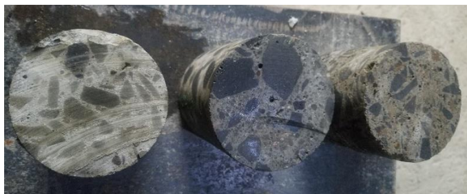
Figure 5.18. Core samples after Trimming from 1 st control mix site
