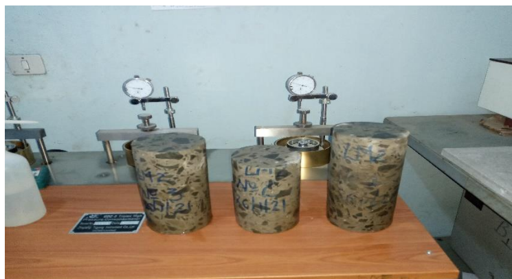
Figure 5.15. Core samples after Trimming from MKB site
