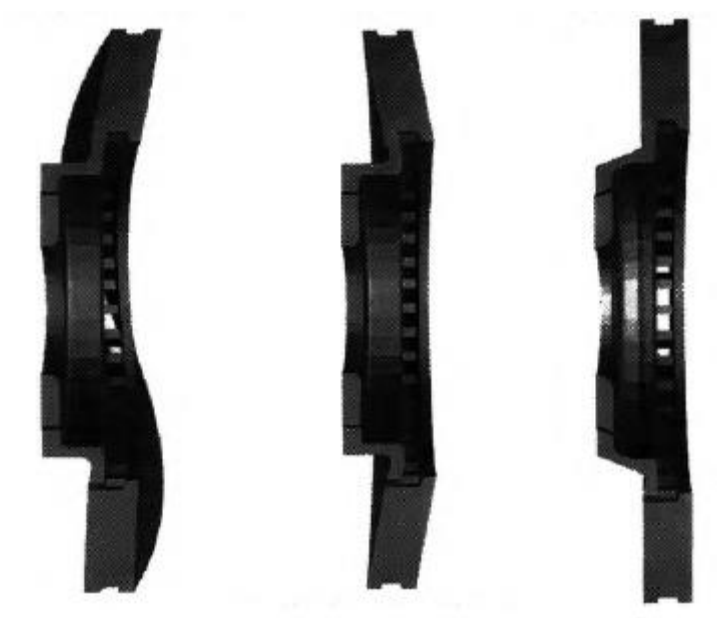
Figure.2.3 Principal distortion types(Waving, Coning and Radial expansion)
