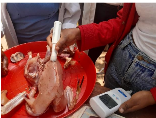
Appendix B 3. Picture of Meat pH measurement after 45 min of post-Slaughter
