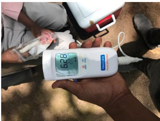
Appendix B 4. Picture of Meat pH measurement after 24 hours of post-Slaughter
