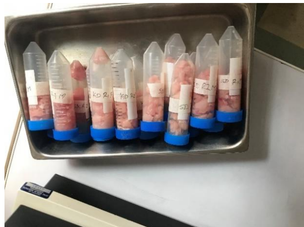
Appendix B 6 . Picture of Water Holding Capacity (WHC) determination of meat using Centrifugal method
