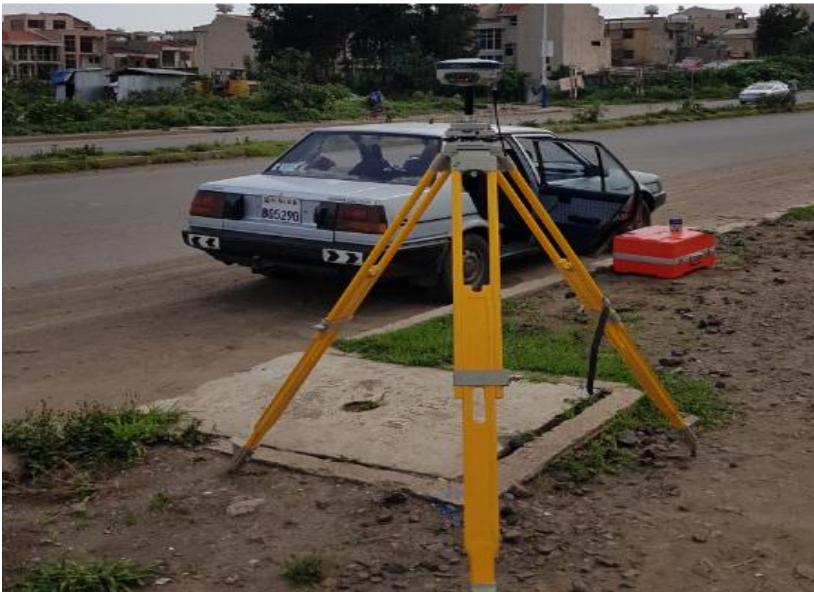
Figure 4.5 - Static GPS observation at one of the twenty CP's location
