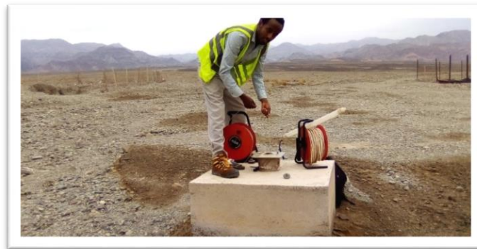
Figure 41. Groundwater level measurement on AY-MO1 (monitoring well).
