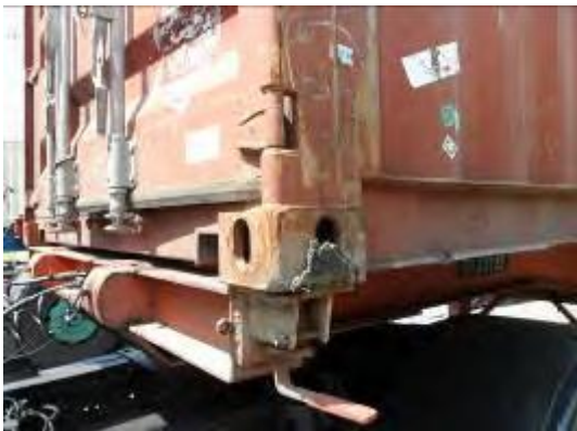
Figure 14: Mud in corner fitting [13]
