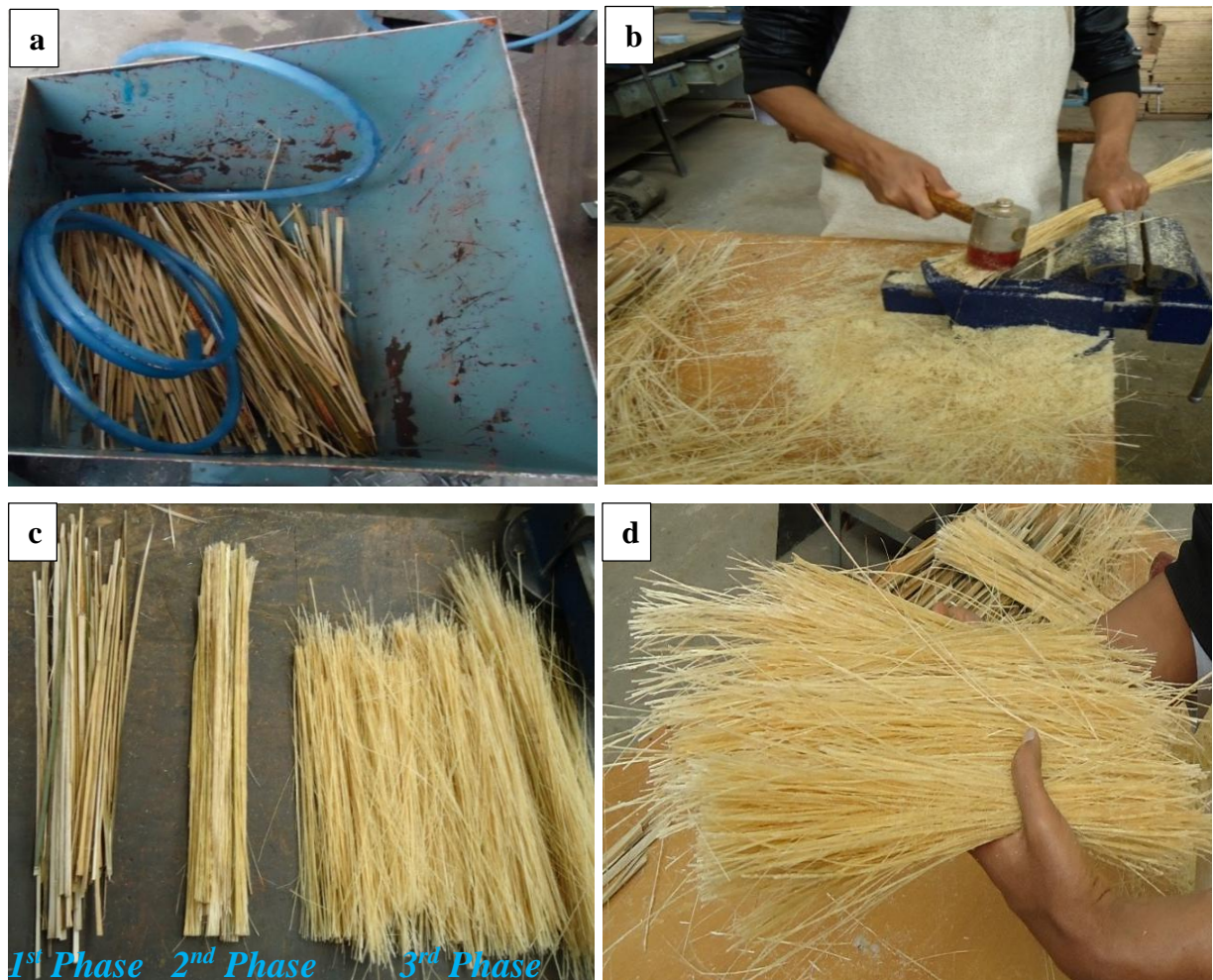
Figure 3.1: Manual extraction process of bamboo fiber
