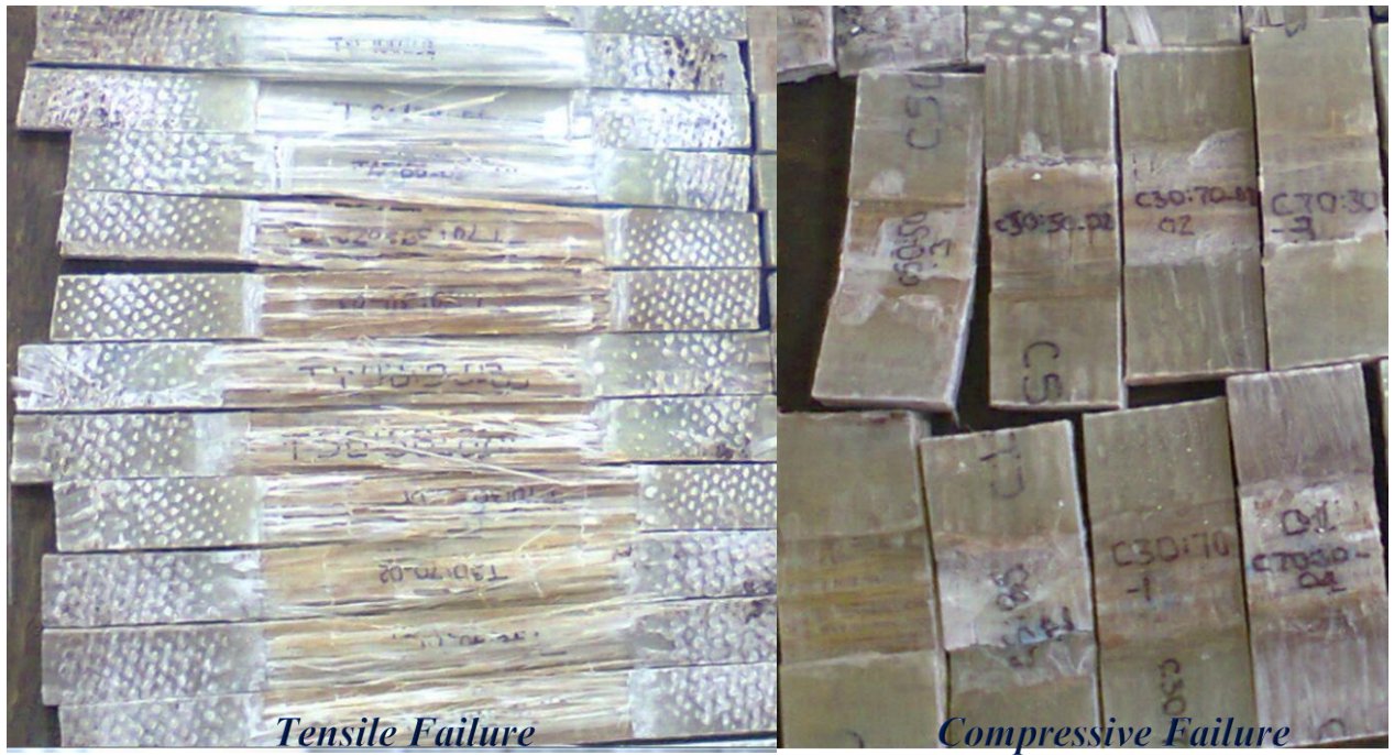
Figure 4.13: Tensile and Compressive failure types
