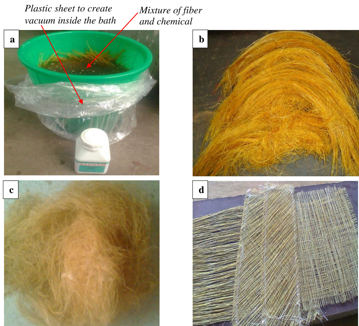
Figure 3.3: Alkaline treatment & mat preparation of bamboo
