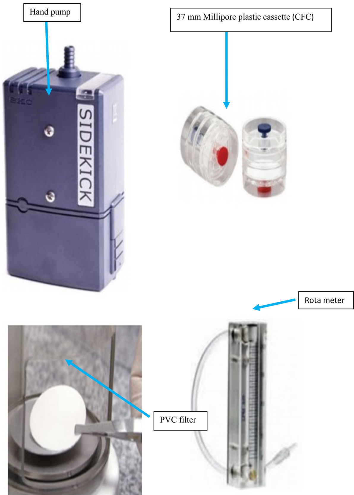
Figure 13: Dust sampling equipments used among woodworkers in Akaki Kality Sub City Addis Ababa 2019.
