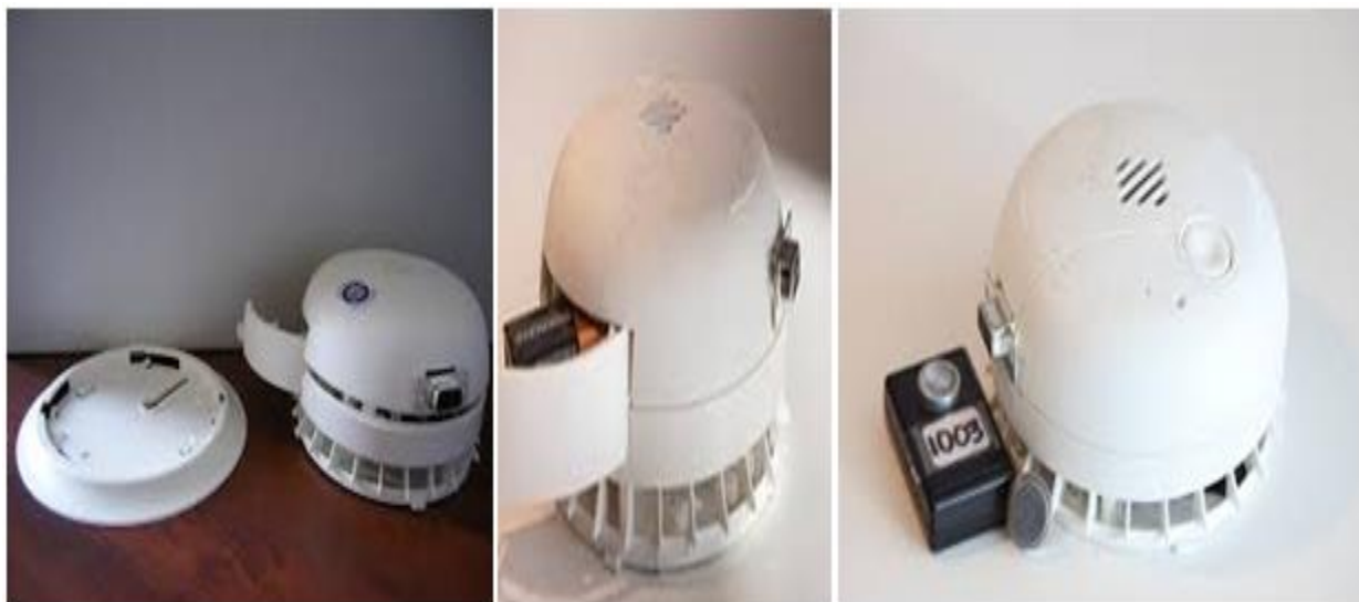
Figure 7. The UCB particles monitor (UCB-PM) used to monitor PM_{2.5}
