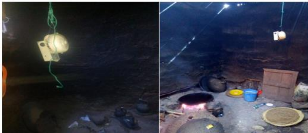
Figure 10. Installing positions of UCB PM and HOBO CO data logger in biomass fuel users
