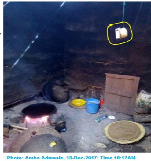
Figure 9. Placement position of UCB PM and HOBO CO data loggers in the kitchen area
