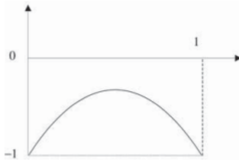
Fig. 3.1. The solution of -u'' + u = 0 in (0, 1) , u(0) = u(1) = -1
