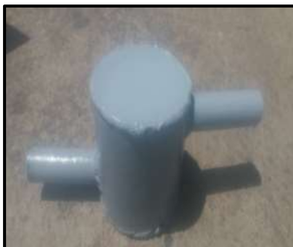
Figure 42: Bed Gas Drier Housing
