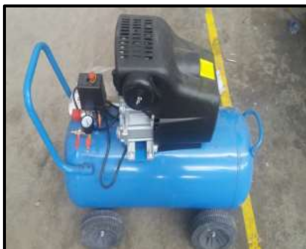
Figure 44: Compressor for Air Supply
