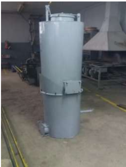
Figure 37: The Gas Production Unit (Gasifier)
