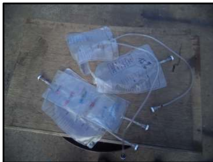
Figure 50: Well Evacuated Gas Sampling Bags (Kits)
