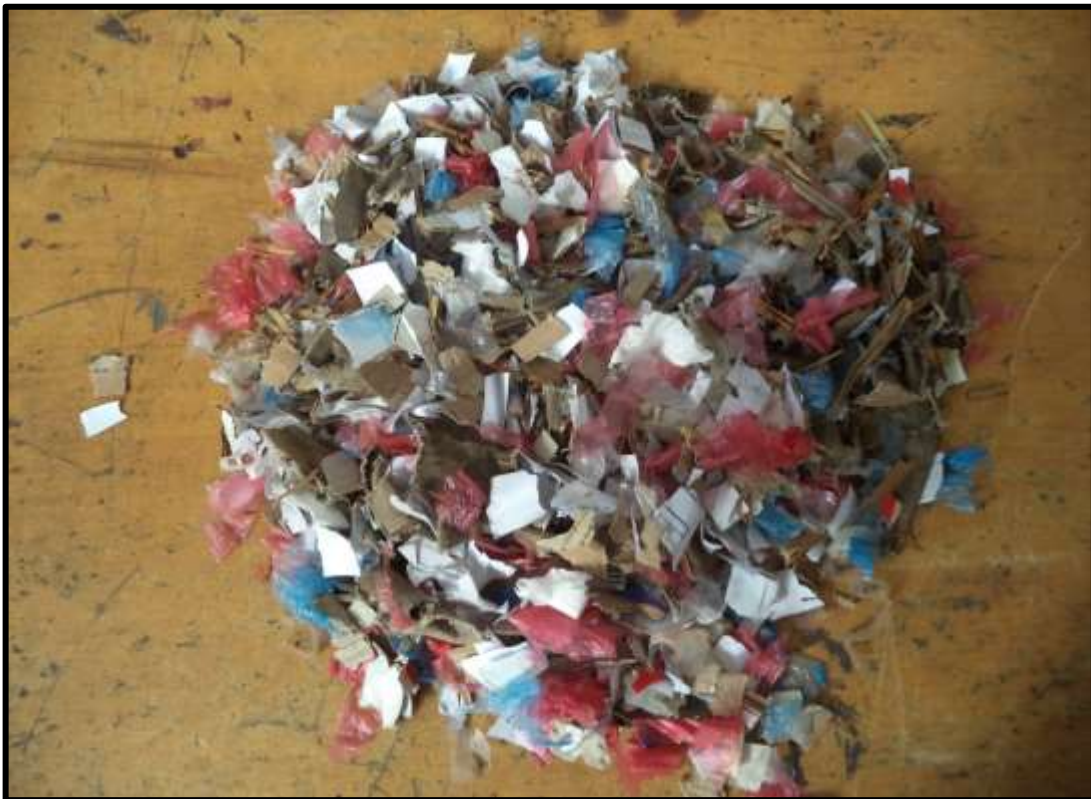
Figure 15: Separated, Dried, Screened and Palletized Waste Sample
