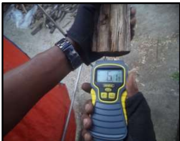
Figure 48: Moisture Content in the Biomass Fraction
