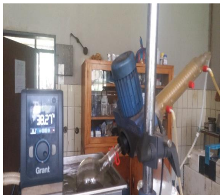
Figure C-7: Vacuum Evaporation of ethanol from the hydrolyzed sample
