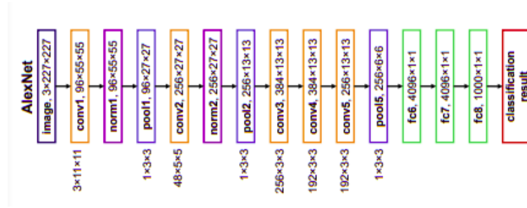
Figure 6.1: AlexNet Hardware configuration to change convolution layer to FC kayer
