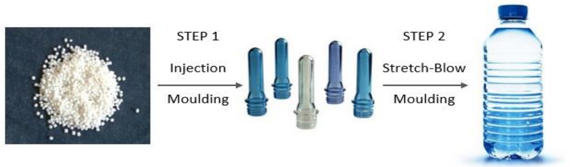
Figure 8 Production Process of Plastic Bottle
