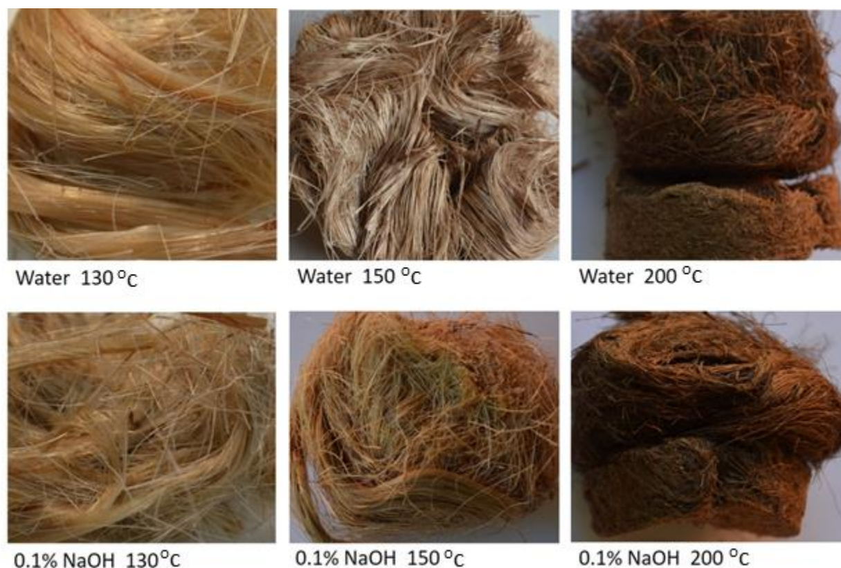
Figure 5. 2: Macroscopic appearances of the Enset fiber bundles after the un-catalyzed hydrothermal treatment and alkali-catalyzed (0.1% NaOH) hydrothermal treatment at 130°C, 150°C, and 200°C
