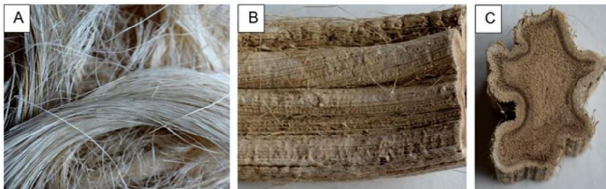
Figure 3.1: Enset fiber bundle (A), longitudinal view of stalk (B) and cross sectional view of stalk (C)
