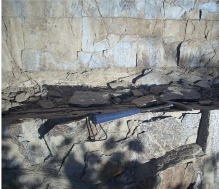
Fig.3.9. Phyllite rock in the field showing shiny cleavage surface with spotty texture
