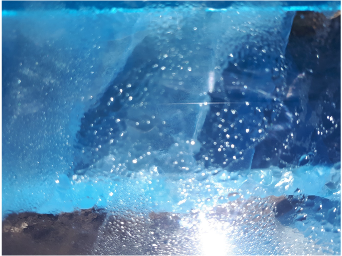
Figure 4-4: Picture of water condensation on inner surface of the glass
