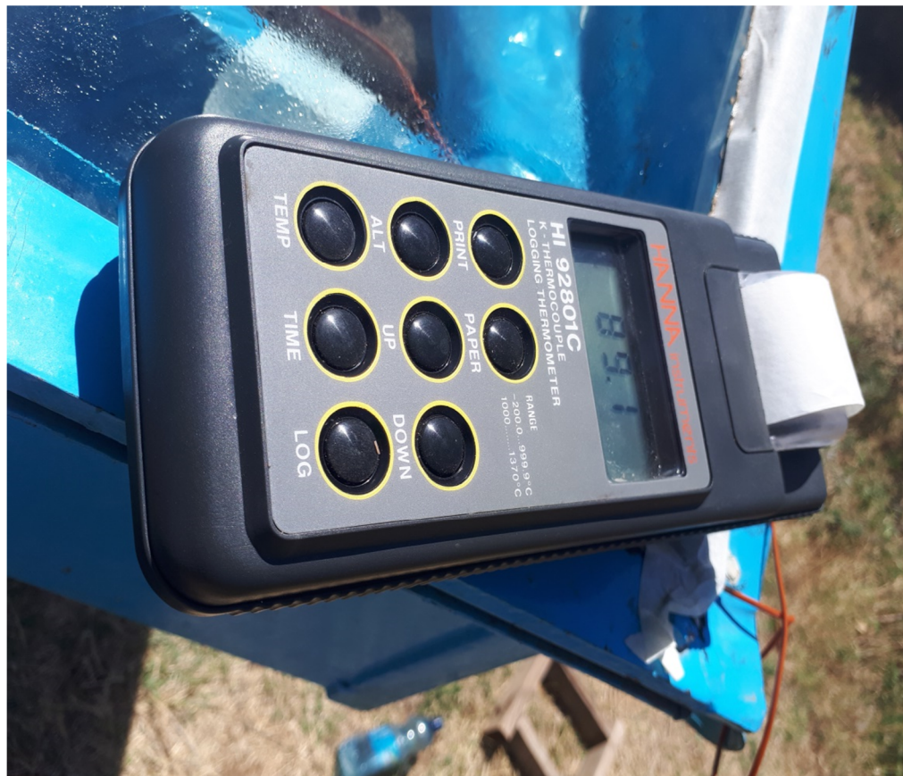
Figure 4-2: HI 92801C K-Thermocouple [le picture during test
