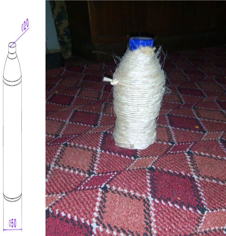
Figure 3-15: Plastic bottle wrapped with Jute
