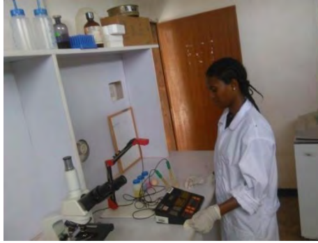
Fig 2: Measuring pH of albumen and yolk by using pH meter
