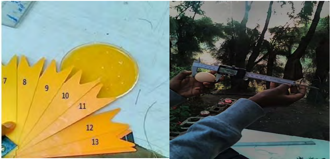
Fig 1: Yolk color determination by Roche color fan (left) and measuring egg length by digital micrometer (right)
