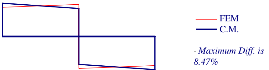
Figure 3-11: Shear Force Diagram for Span ratio 2.0 and BC = 9.
