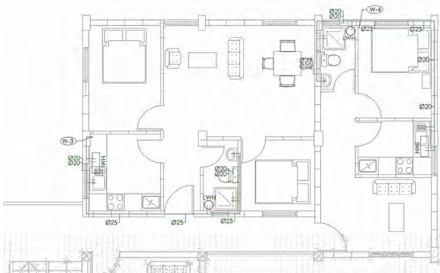
Figure 4-2 Typical water supply system in a condominium typology
