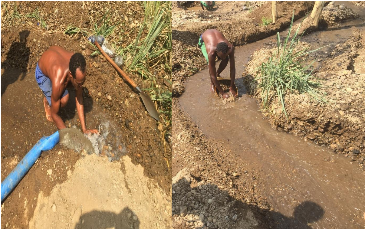
Figure 24 Ground sluicing for gold recovery
